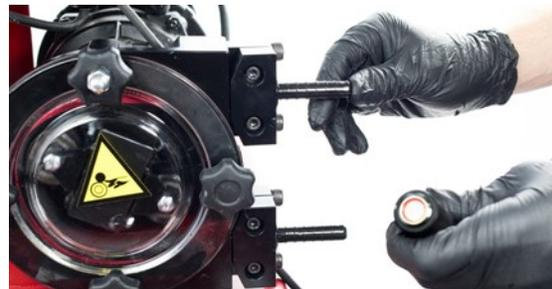
**STEP 6** ▶ Cut a 1.3m / 4.3ft of orange resin supply hose. Piece needs to be long enough to reach from the resin cup to the top hose connector. Connect to the top hose connector and secure with a hose clamp. Guide the other end through the guide holes and place in resin supply cup. Be sure there is a 45° cut on the end placed in the resin supply cup to allow for proper resin flow into the hose.
