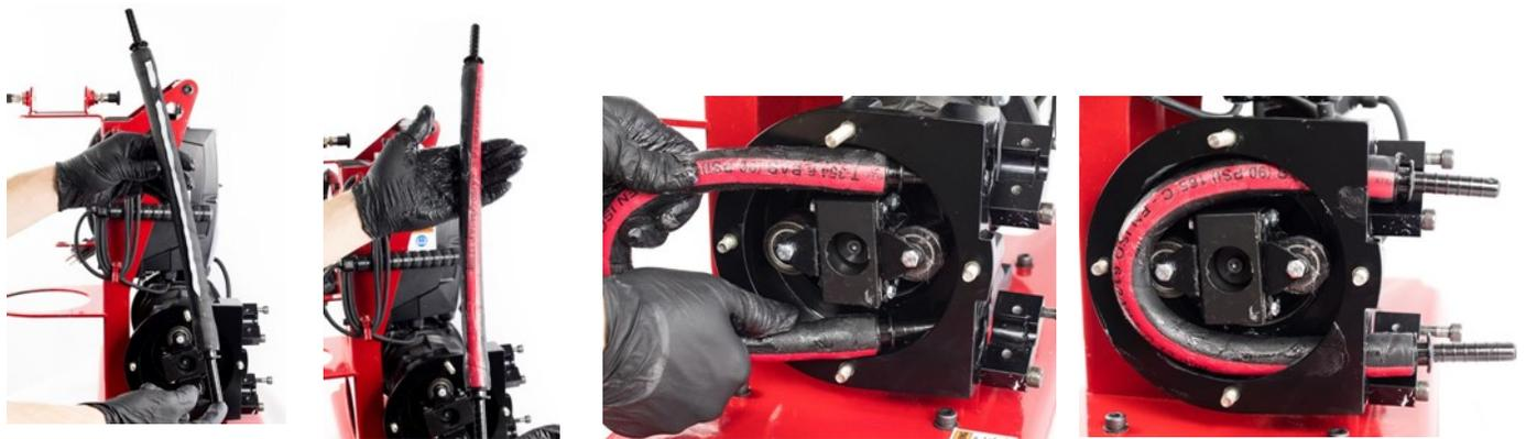
**STEP 3** ▶ Next reinstall and tighten the locking blocks making sure the pump hose connectors are positioned properly. Note: The locking block should fit into the groove on the hose connector.
