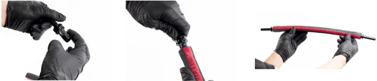
**STEP 2** ▶ Once the pump hose is assembled, apply silicone grease to the outside. Then place the hose into the pump housing. Note: Do not insert hose into the roller assembly at this time.
