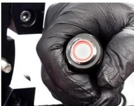
This machine has a hand-held locking operator control bottom or "LOC". When the control button is pushed the pump is engaged and will operate until depressed.
