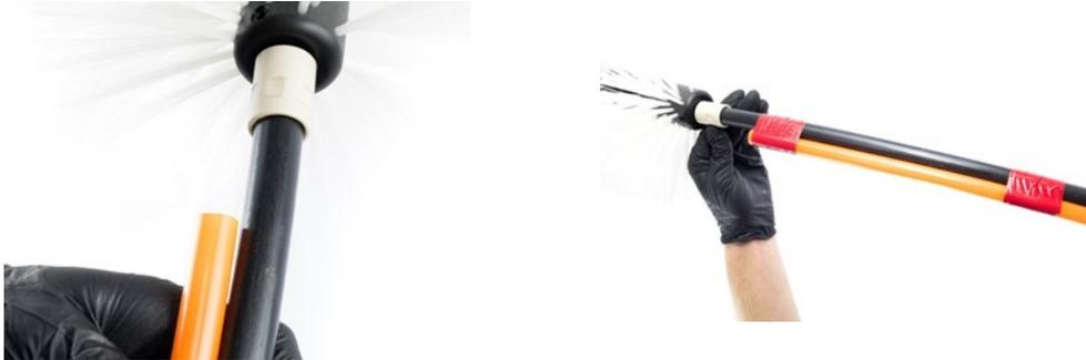
**STEP 4** ▶ Using your camera screen, position and attach the camera 100mm to 200mm / 4" to 8" behind the delivery hose ensuring the rear brush is visible in the camera monitor. In pipes DN100 / 4" and larger, it is recommended to tape the entire camera head and spring for easier cleanup. In smaller pipes it is recommended to leave the spring of the camera untaped in order to retain flexibility.
