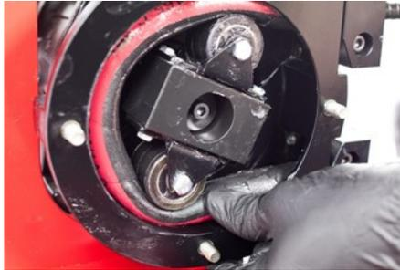
**STEP 5** ▶ Place the cover plate back on the pump housing, ensuring the cover is flush and can be secured evenly all around. Set the pump speed dial to full speed and test for proper suction by placing a finger over the end of the top hose connector. Positive suction should be obvious. If no suction is present the mounting blocks may need to be secured more tightly.
